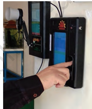
Fig. 4.9: Aadhaar-enabled biometric attendance system
