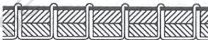
Fig. 2.43: Seams when the upper tension is too tight
